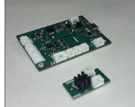
Figure 7: Assembled PCB Boards
